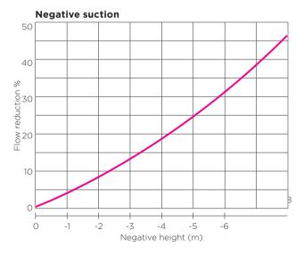
Lifting the liquid from a negative height reduces the flow of the pump as in standard circumstances (flooded suction).
